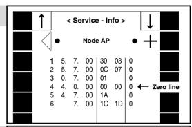
If the zero line is in line 1, the queried node (PCB) is in order electrically.
