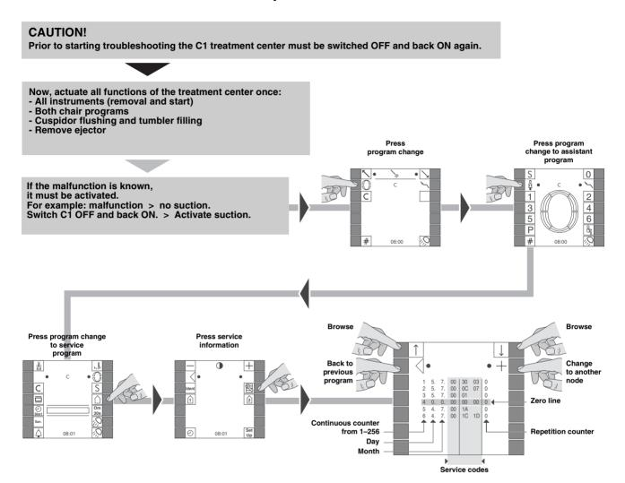
Only the service codes above the zero line must be taken into account for troubleshooting. The most up-to-date service code can be found in line 1.
